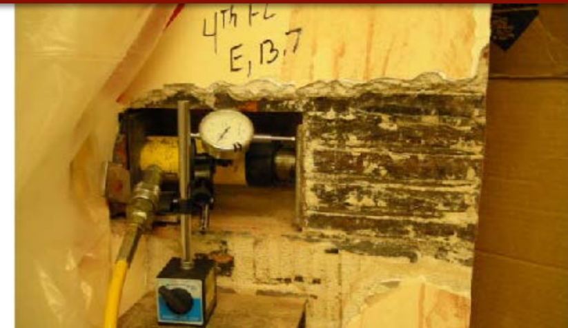
In Situ shear strength of wall element
